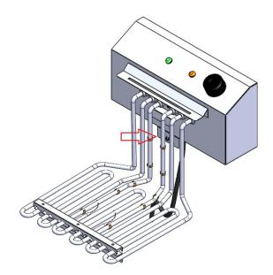
Note that the immersion level must not be exceeded, otherwise the equipment may be damaged or even the user may be endangered.
