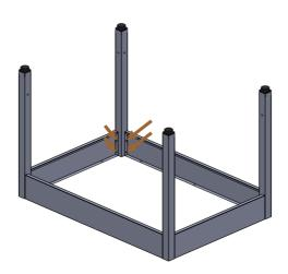
3. Apply the back and side rails as shown in the picture (apply 6 M6 screws);
