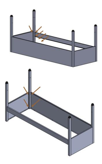
2º Apply the plug and screw it underneath (Screw M6);
